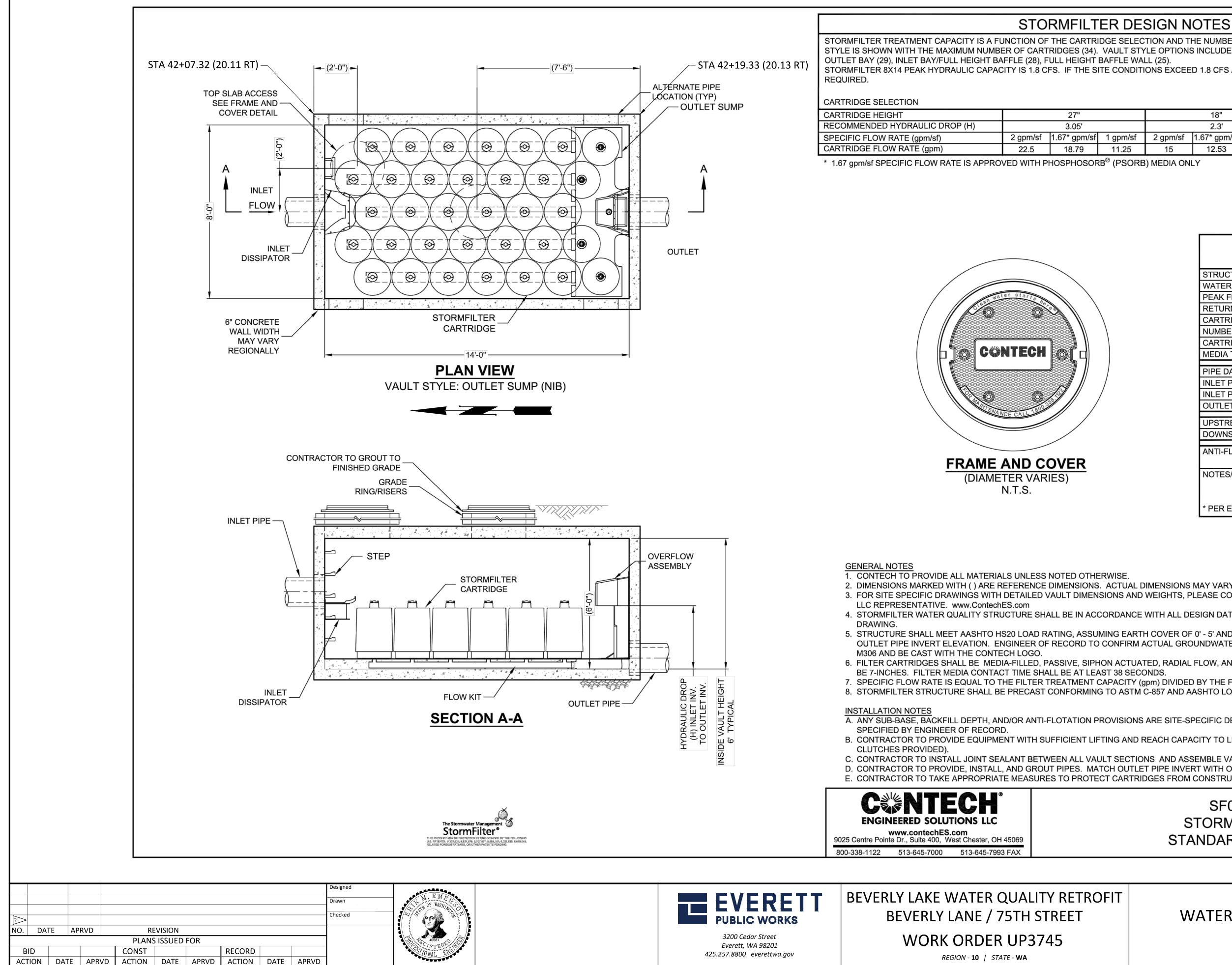
STORMFILTER TREATMENT CAPACITY IS A FUNCTION OF THE CARTRIDGE SELECTION AND THE NUMBER OF CARTRIDGES. THE STANDARD VAULT STYLE IS SHOWN WITH THE MAXIMUM NUMBER OF CARTRIDGES (34). VAULT STYLE OPTIONS INCLUDE INLET BAY (27), INLET BAY/OUTLET BAY (22), OUTLET BAY (29), INLET BAY/FULL HEIGHT BAFFLE (28), FULL HEIGHT BAFFLE WALL (25). STORMFILTER 8X14 PEAK HYDRAULIC CAPACITY IS 1.8 CFS. IF THE SITE CONDITIONS EXCEED 1.8 CFS AN UPSTREAM BYPASS STRUCTURE IS
