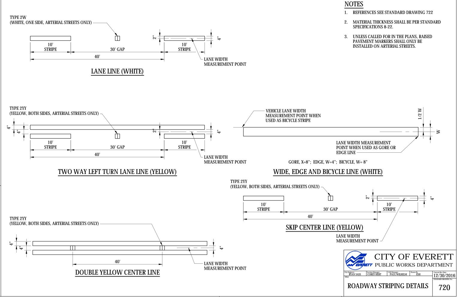
menne Marcad Leps-COE DESIGN & CONSTR SPECS FOR DEVELOPMENT/IN-WORK/STD720.DWG PLOTTED: 1/25/2019 1:24 PM
